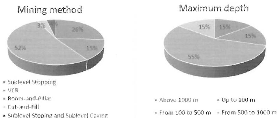
Figure 1. Distribution of mines according to the mining method and maximum depth
